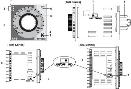
1. Deviation indicator: It shows deviation of present temperature (PV) based on set temperature (SV) by LED.
