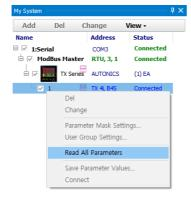
12. It is possible to check the progress for 'read parameters' at the bottom of the model in 'Add' row of the 'My System' control panel. Checking and setting parameter values is available in the 'Property' control panel.
