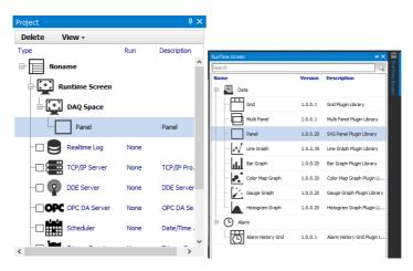
9. Drag the I/O source to be monitored from the 'DAQ List' and drop it onto the RunTime Screen.
