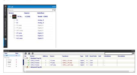
8. For visualized monitoring, double-click the desired runtime screen in the 'RunTime Screen' and import to 'DAQ Space'. Imported runtime screen is displayed in the 'Project' control panel as well.
