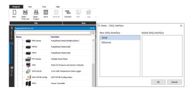
3. Proper communication port setting is needed to connect the device. Select Serial in 'My System' control panel. In 'Property' control panel, click pull-down icon ▼ on 'communication port' and select the communication port currently in use.
